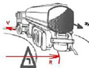
Whenever the relationship of speed and radius to the curve provides an acceleration above 0.3 g's (and there isn't any correction of a superelevation) overturning will occur frequently at this point.
