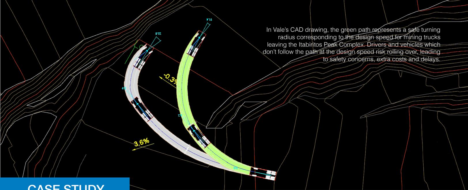
In Vale's CAD drawing, the green path represents a safe turning radius corresponding to the design speed for mining trucks leaving the Itabiritos Peak Complex. Drivers and vehicles which don't follow the path at the design speed risk rolling over, leading to safety concerns, extra costs and delays.
