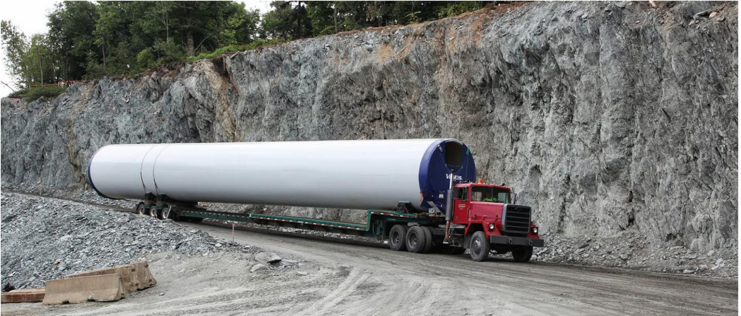
Companies like Green Mountain Power use AutoTURN to plan exact routes with the large wind farm components, reducing costs for blasting and excavating bedrock.
