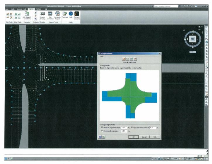
number, type and position of entry and exit lanes. All options are shown in a preview of the junction and then applied to the drawing directly.
