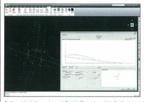
As the vertical alignments are defined in Nexus, immediate feedback on the cross slopes is graphically shown on the plan and profile view.
